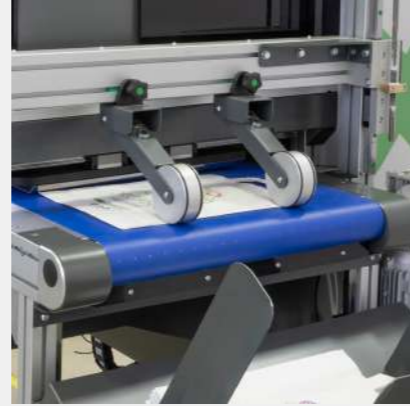
OUTLET PRESSURE ROLLERS
